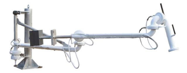
This type of loading arm is especially designed to load LNG products. It is suitable for the bottomloading/unloading of Road or Rail tankers. The loading arm has a long reach and is suitable for applications where tanker connection flange cannot be accurately positioned.
