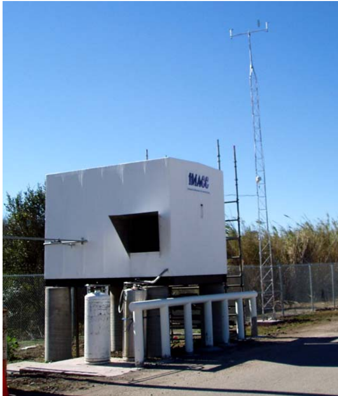
Imacc Instrument shelter for open-path FTIR monitor
