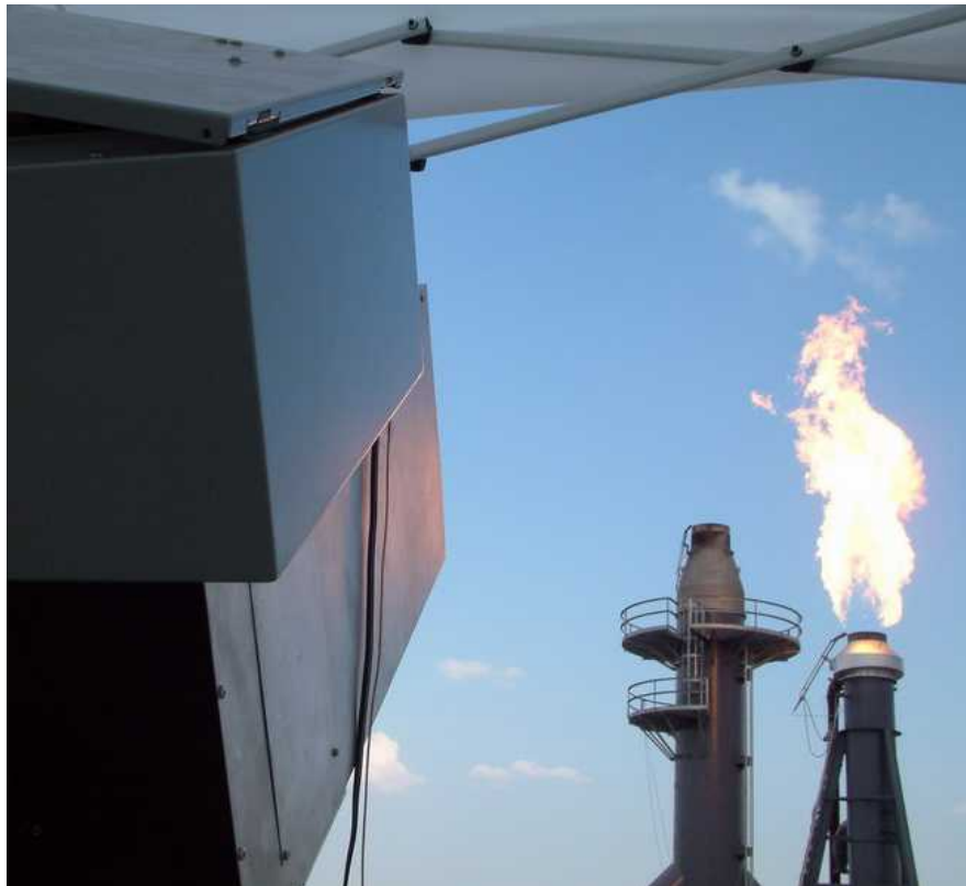
Imacc Passive Radiometer system under testing by Texas Commission on Environmental Quality at John Zink facility in Oklahoma
