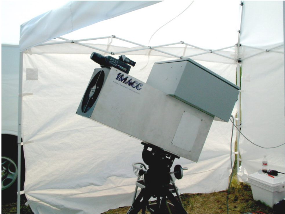
Imacc Passive Radiometer for use in stack/flare monitoring
