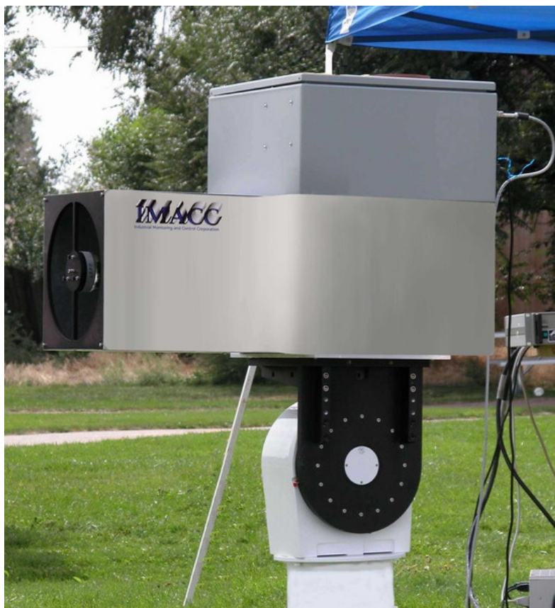
Imacc Monostatic FTIR Open-Path Monitor on motorized Az/EI mount in use by EPA at a toxic waste site
