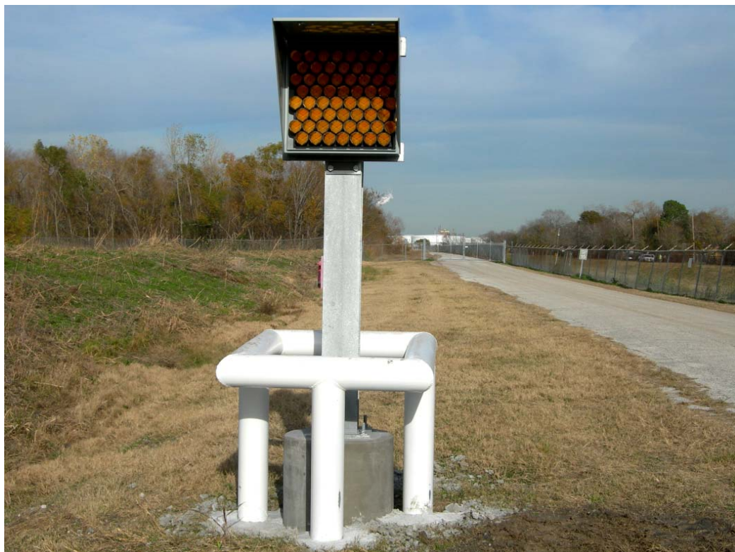
Array of corner cube mirrors used to direct the FTIR beam back to the transmitting telescope.
