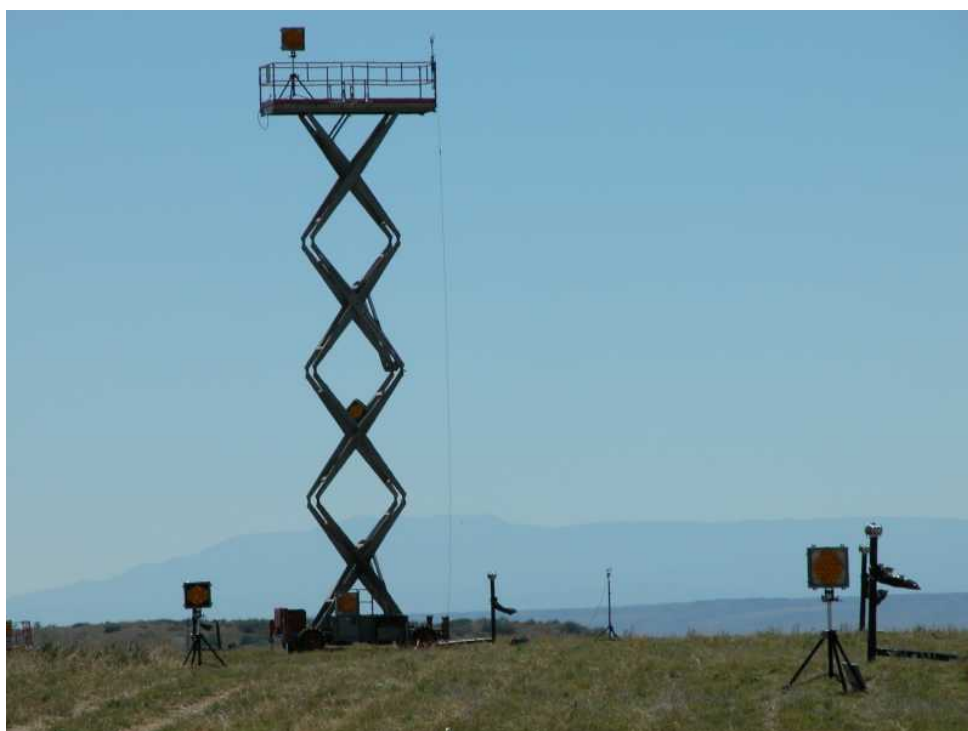
Corner-cube arrays used in waste site monitoring by US EPA
