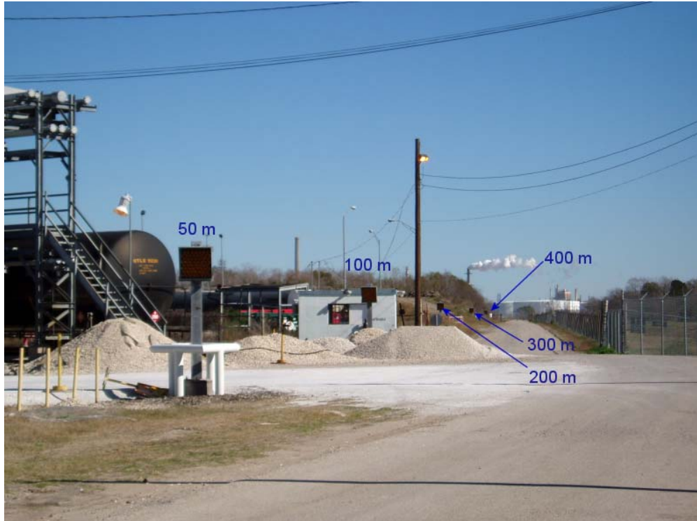
Retro mirrors set up along the South boundary of Texas Petrochemicals at 50m, 100m, 200m, 300m, and 400m.
